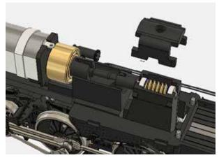
Using a small flat head screwdriver, pry off the worm gear cover, exposing the worm gear. At this point, you can service the motor by de-soldering the leads and replacing or changing. Please note that changing any electronics in your locomotive will void your warranty.
