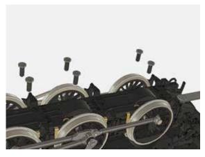
On the bottom of your locomotive, there are a series of 6 (six) screws that secure the gear cover on. Placing the locomotive on a secure work station, such as a foam cradle, remove these screws. Place these screws somewhere where you will not lose them. A small dish or container is suggested to hold these screws and stop them from rolling off your work station.
