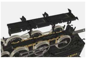
After you have removed the screws and placed them in a safe location, lift off the GEAR COVER. Lift the cover STRAIGHT UP taking care not to damage the moulded brake supports. This will expose the IC and PICK-UPS and 6 more screws. Remove these 6 (six) screws and the IC and PICK UPS. Please take notice: DO NOT BEND THE ELECTRICAL PICK UPS! Creasing or crimping them will result in erratic pickup.
