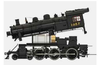
Tilting the boiler from the BACK forward (as depicted in the illustration) slide the boiler off. This will leave exposed the motor, universal, worm gear cover, and flywheel. Place the boiler in a safe place where not damage will occur.
